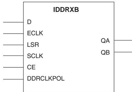
Table 10-6 provides a description of all I/O ports associated with the IDDRXB primitive.
