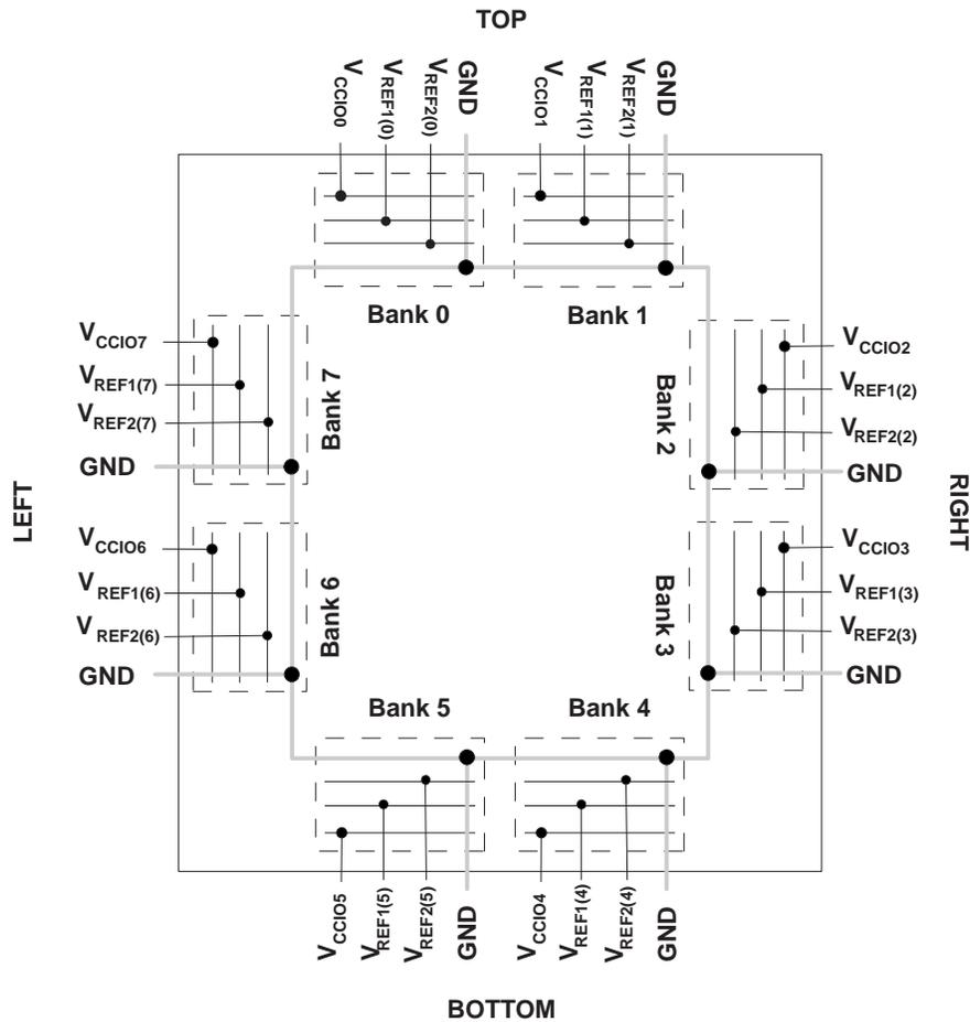
LatticeECP/EC devices contain two types of sysI/O buffer pairs.
