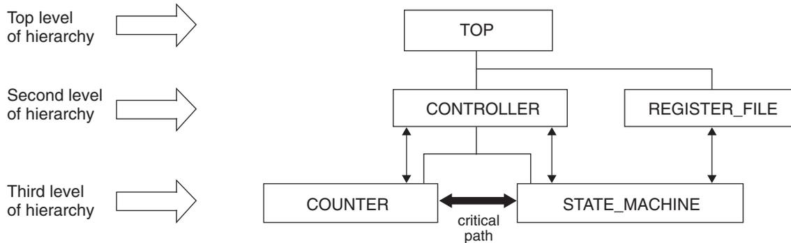
Figure 17-3 illustrates a design hierarchy where the failing paths are the connections between COUNTER and STATE\_MACHINE design blocks. The easiest implementation for this example is to PGROUP the CONTROLLER, which is the module in which the COUNTER and STATE\_MACHINE are instantiated within.
