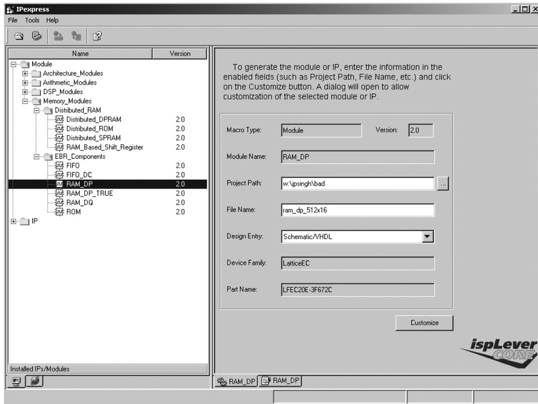
In the right-hand pane, options like **Macro Type**, **Version**, and **Module\_Name** are device and selected module dependent. These cannot be changed in IPexpress.
