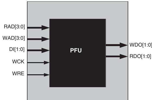
Ports such as Read Clock (RdClock) and Read Clock Enable (RdClockEn) are not available in the hardware primitive. These are generated by IPexpress when the user wants to enable the output registers in the IPexpress configuration.
