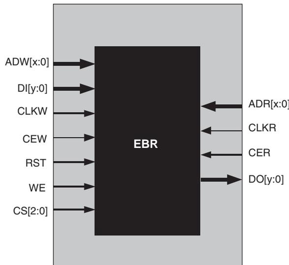
In the Pseudo Dual Port RAM mode, the input data and address for the ports are registered at the input of the memory array. The output data of the memory is optionally registered at the output.
