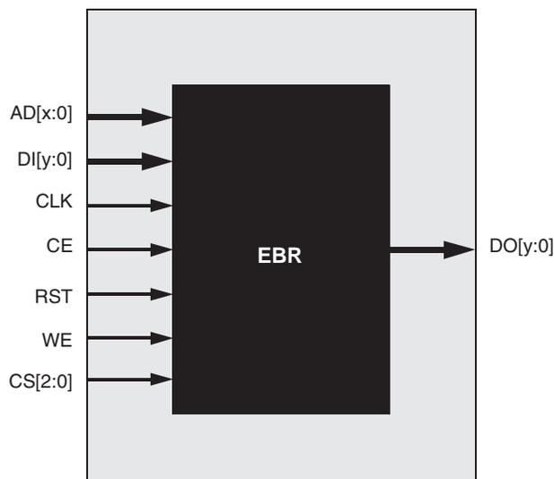
In Single Port RAM mode the input data and address for the ports are registered at the input of the memory array. The output data of the memory is optionally registered.
