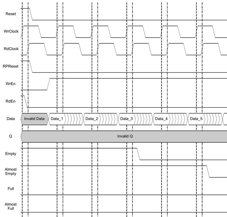
**Figure 9-47. FIFO\_DC With Output Registers, End of Data Write Cycle**
