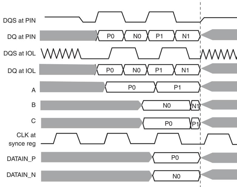
LatticeECP/EC and LatticeXP devices have extra dedicated logic in the in the DQS Delay Block that will prevent this postamble problem. The DQS postamble logic is automatically implemented when the user instantiates the DQS Delay logic (DQSBUFB software primitive) in a design.
