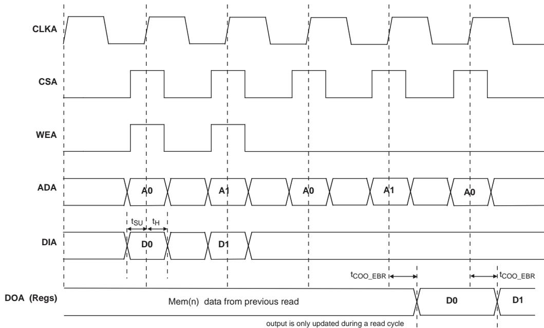
Figure 3-10. Read Before Write (SP Read/Write on Port A, Input Registers Only)
