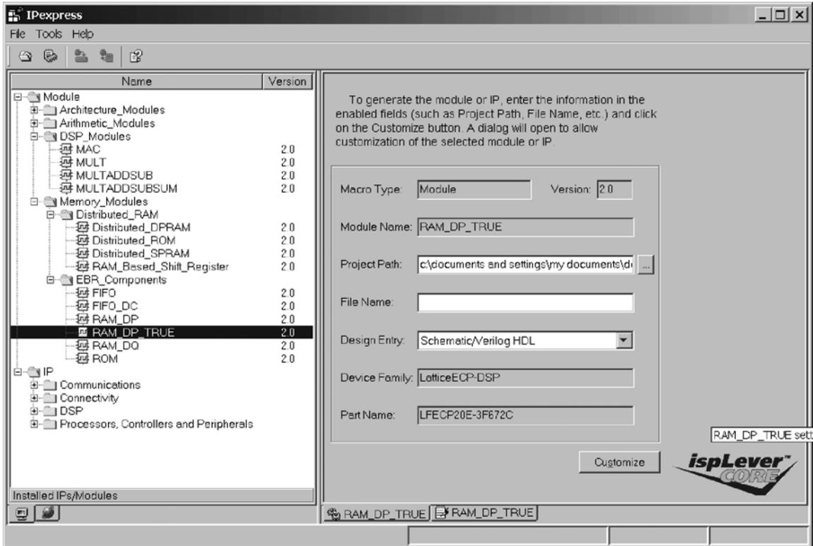
When implementing large memories in the design, it is recommended to construct the memory from the Enhanced Block RAM (EBR) components found in every Lattice Semiconductor FPGA device. When implementing small memories in the design, it is recommended to construct the memory from the resources in the PFU. The memory utilizing resources in the PFU can also be generated by IPexpress.
