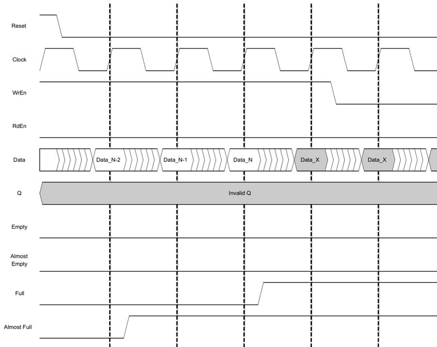
In this case, as seen above, the Almost Full flag is IN location 2 before the FIFO is filled. The Almost Full flag is asserted when N-2 location is written, and Full flag is asserted when the last word is written into the FIFO.
