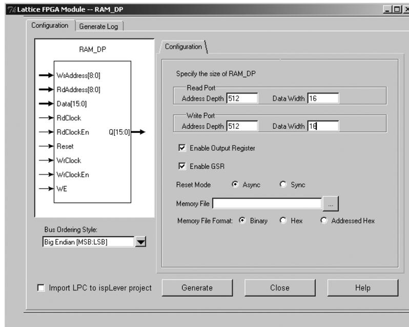
Users can specify the Address Depth and Data width for the **Read Port** and the **Write Port** in the text boxes provided. In this example we are generating a Pseudo Dual Port RAM of size 512 x 16. Users can also create RAMs of different port widths in the case of Pseudo Dual Port and True Dual Port RAMs.
