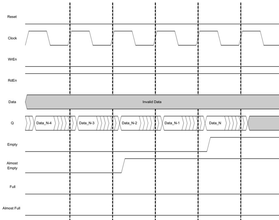
Figures 9-33 to 9-36 show the behavior of non-pipelined FIFO or FIFO without output registers. When we pipeline the registers, the output data is delayed by one clock cycle. There is an extra option of output registers being enabled by RdEn signal.
