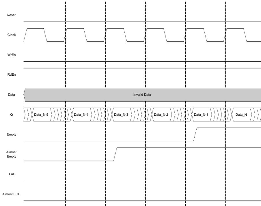
And finally, if you select the option enable output register with RdEn, it still delays the data out by one clock cycle (as compared to the non-pipelined FIFO), and the RdEn should be high also during that clock cycle, otherwise the data takes an extra clock cycle when the RdEn goes true.
