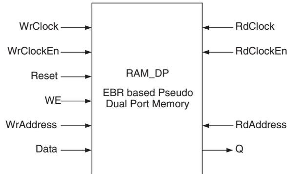
The generated module makes use of these EBR blocks or primitives. For memory sizes smaller than an EBR block, the module will be created in one EBR block. If the specified memory is larger than one EBR block, multiple EBR block can be cascaded, in depth or width (as required to create these sizes).
