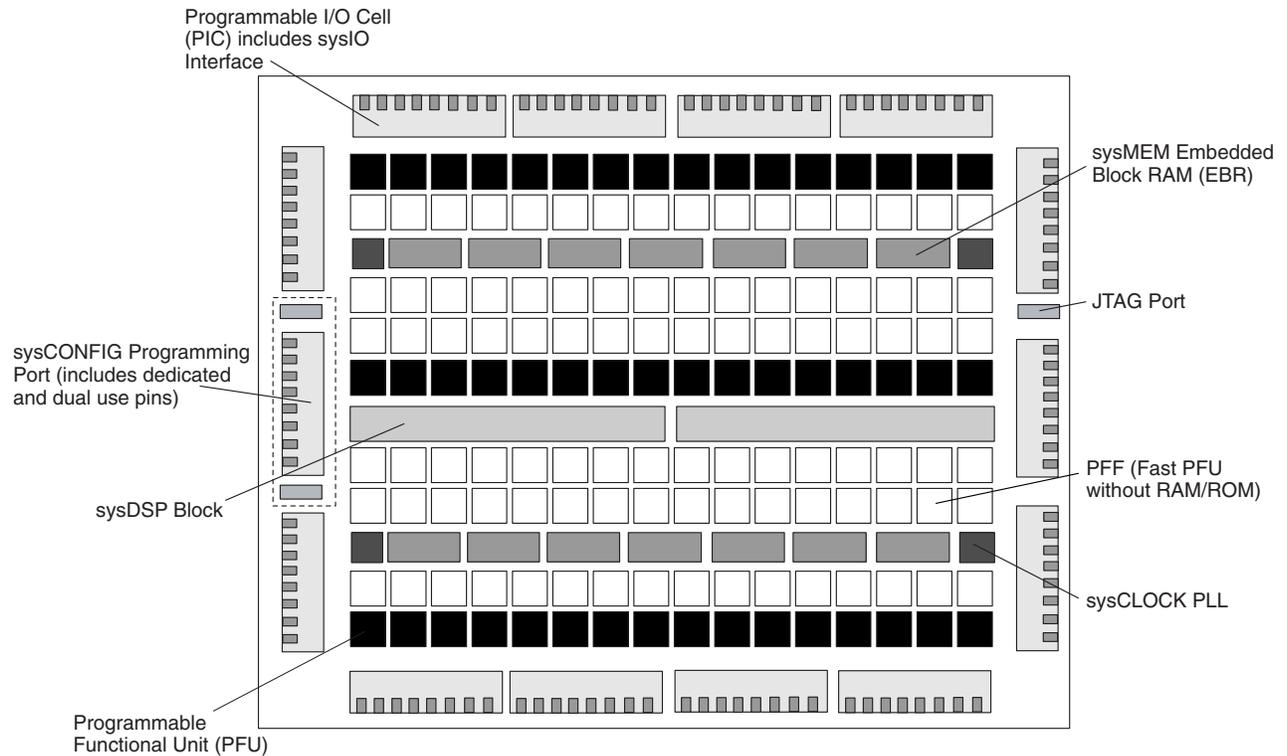
Figure 9-3. Simplified Block Diagram, LatticeXP Device (Top Level)
