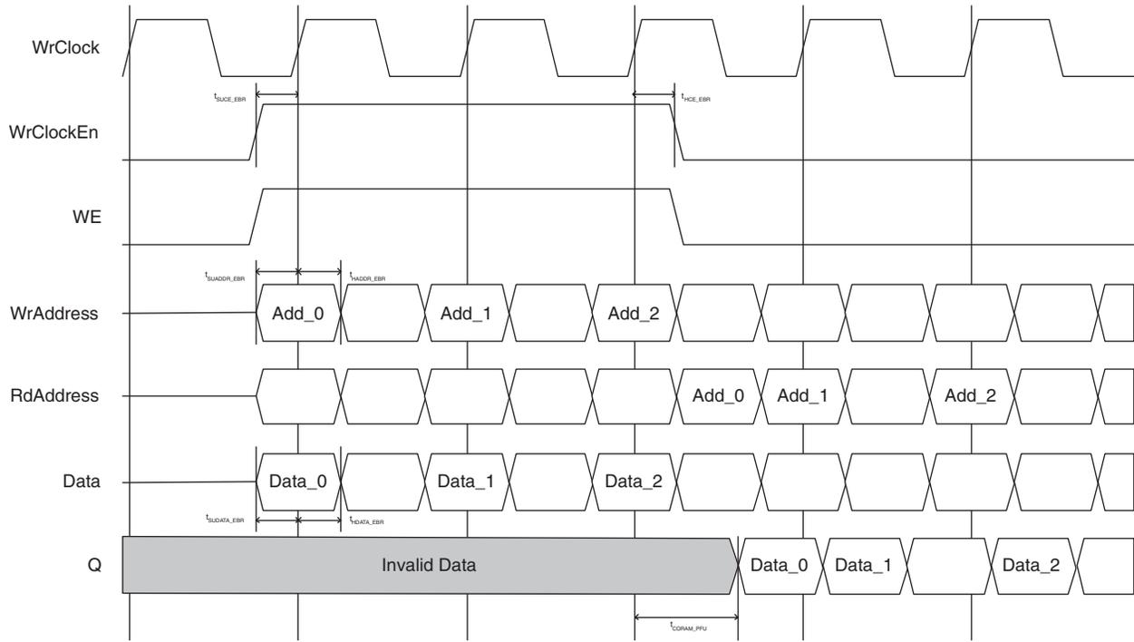
Figure 9-60. PFU-based Distributed ROM (Sync\_ROM) for LatticeECP/EC and LatticeXP Devices
