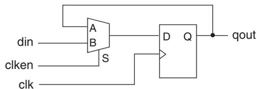
The VHDL and Verilog coding for Clock Enable are as shown in Figure 15-10.
