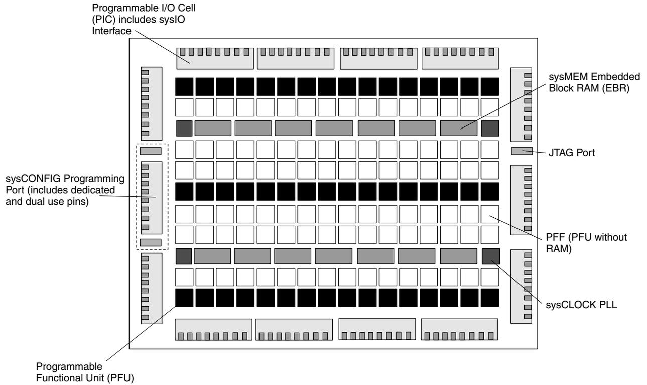
Figure 2-2. Simplified Block Diagram, LatticeECP-DSP Device (Top Level)
