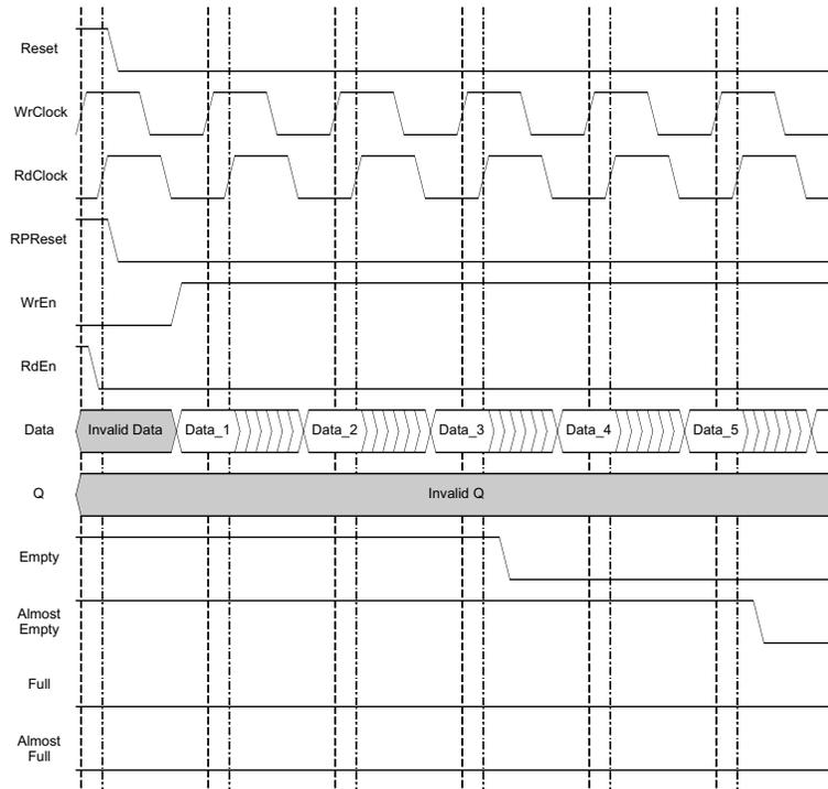
The WrEn signal has to be high to start writing into the FIFO\_DC. The Empty and Almost Empty flags are high to begin and Full and Almost full are low.
