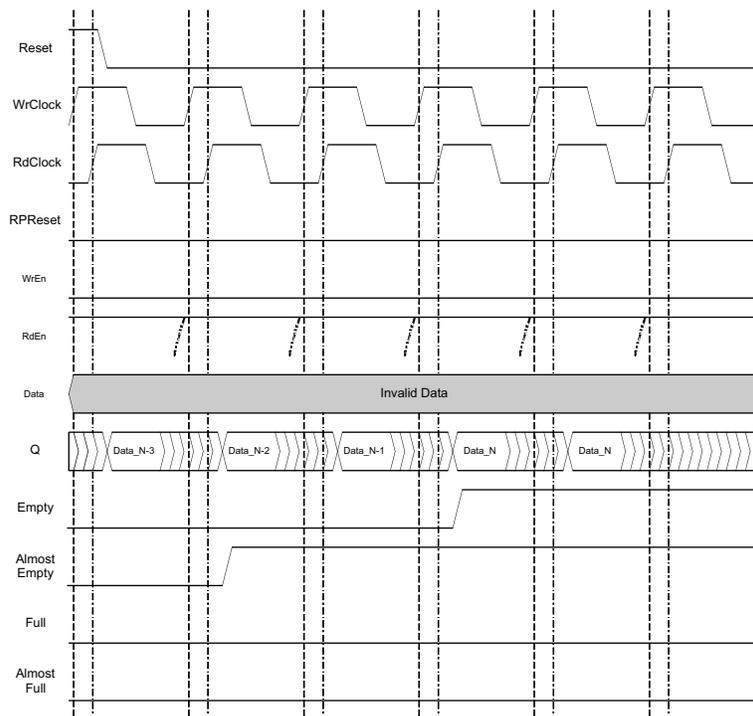
Figures 9-42 to 9-45 show the behavior of non-pipelined FIFO\_DC or FIFO\_DC without output registers. When we pipeline the registers, the output data is delayed by one clock cycle. There is an extra option for output registers to be enabled by the RdEn signal.
