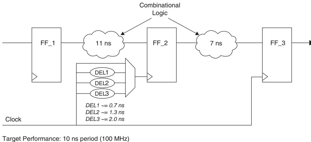
The example illustrated in Figure 16-11 shows two register-to-register transfers that both need to meet the 10 ns period constraint. By using delay cell DEL2 to delay the clock input on flip-flop FF\_2, the first register transfer will make its period constraint with a new minimum period of ~9.7 ns and the second register transfer will make its period constraint by ~8.3 ns.
