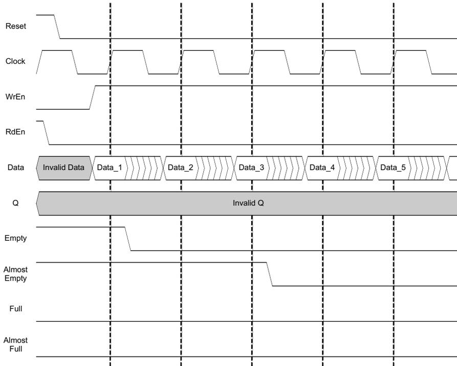
The WrEn signal has to be high to start writing into the FIFO. The Empty and Almost Empty flags are high to begin and Full and Almost full are low.
