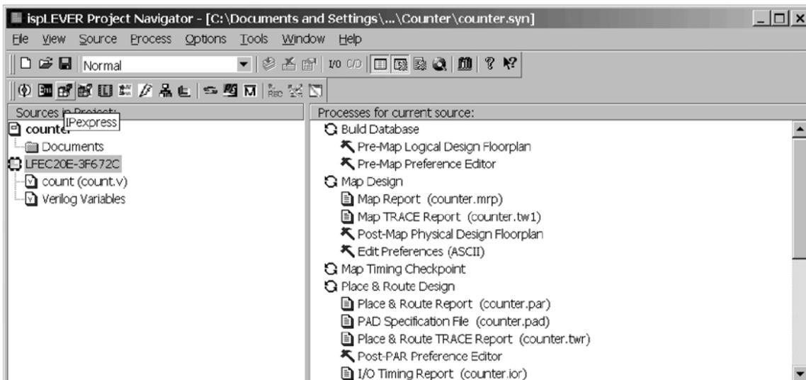
Once IPexpress is launched, you will be presented with the option of generating the ispTRACY IP module by selecting the JTAG module under Architecture and clicking the Customize button. Figure 14-2 shows the IPexpress window. Selections for the project path and module name are made through this window
