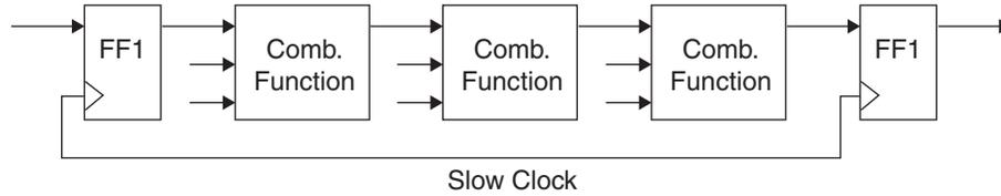
**Figure 15-6. After Pipelining**
