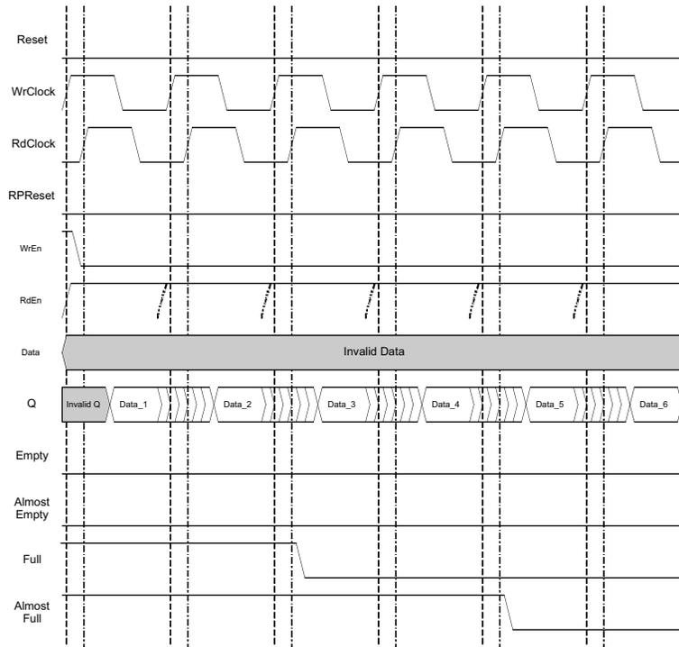
Similarly, as the data is read out and FIFO\_DC is emptied, the Almost Empty and Empty flags are asserted. Below is the
