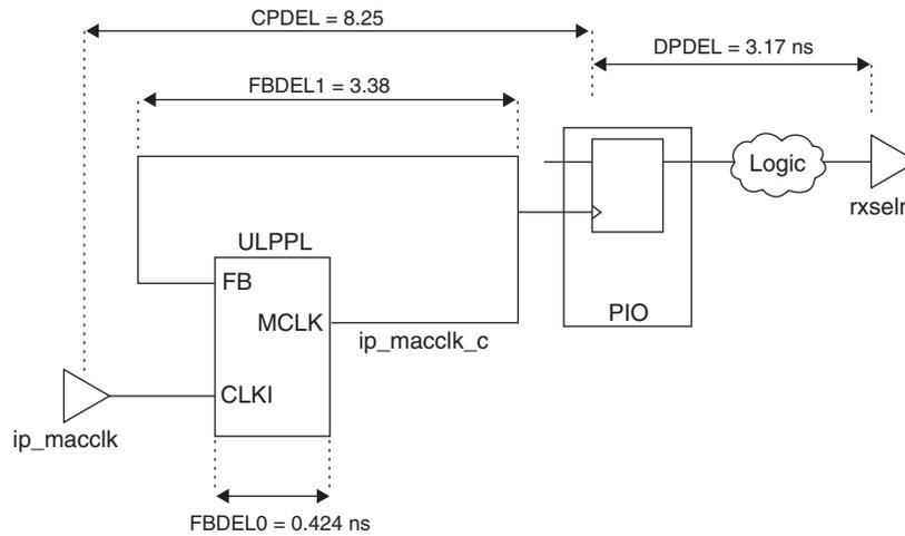
Figure 16-7. Trace Report for CLOCK\_TO\_OUT with PLL
