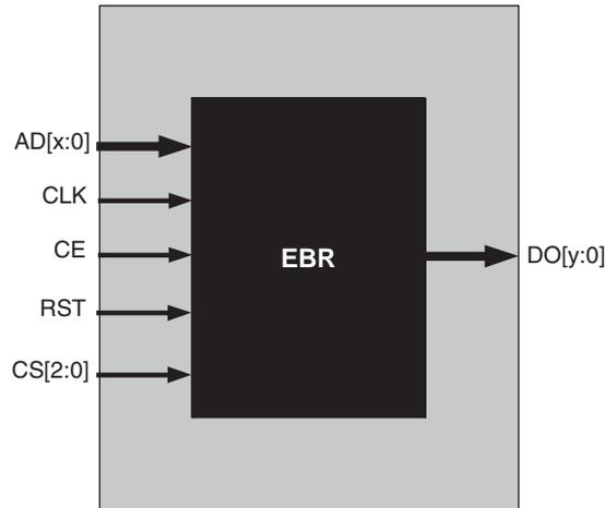
In the ROM mode the address for the port is registered at the input of the memory array. The output data of the memory is optionally registered at the output.
