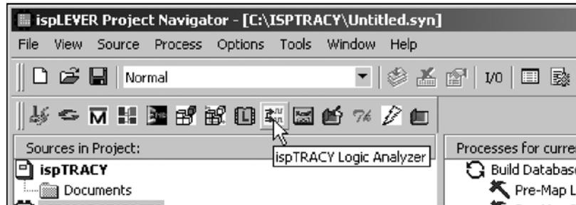
ispLA provides for capture and display of data from the ispTRACY core. The program is used to setup the trigger events counters, trigger location in data buffer, event patterns, event comparisons and data display. Figure 14-8 shows the initial startup windows required to run ispLA.
