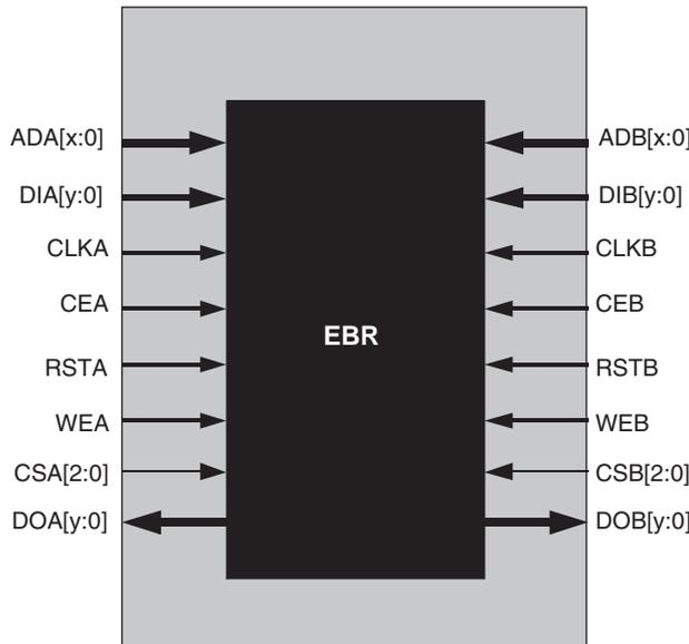
In True Dual Port RAM mode, the input data and address for the ports are registered at the input of the memory array. The output data of the memory is optionally registered at the output.
