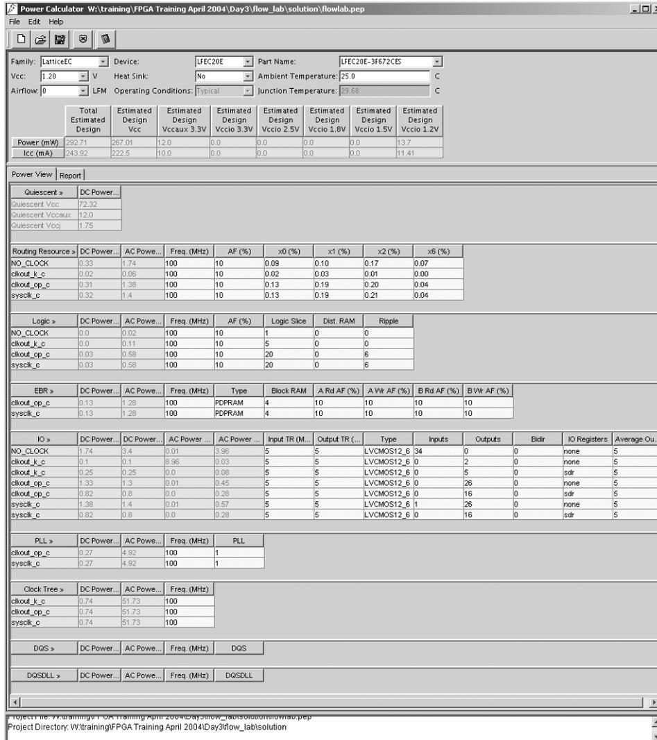
The second and third columns from the left indicate the DC (or static) and AC (or dynamic) power consumption. The total power consumption for the design can be seen in the same table. Scroll down to the row labeled **Total**.
