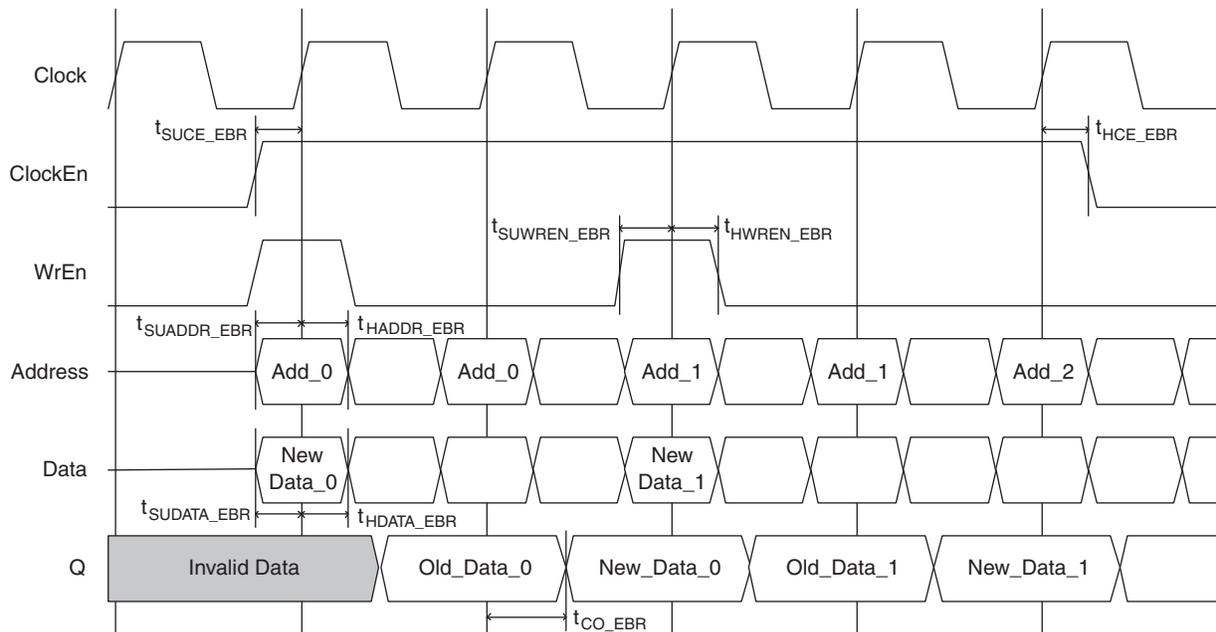
**Figure 9-12. Single Port RAM Timing Waveform – READ BEFORE WRITE Mode, with Output Registers**
