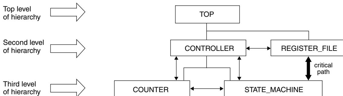
Figure 17-4 shows an example design hierarchy where the failing paths are the connections between REGISTER\_FILE and STATE\_MACHINE modules. The simplest thing to do here is to UGROUP the REGISTER\_FILE and STATE\_MACHINE together.
