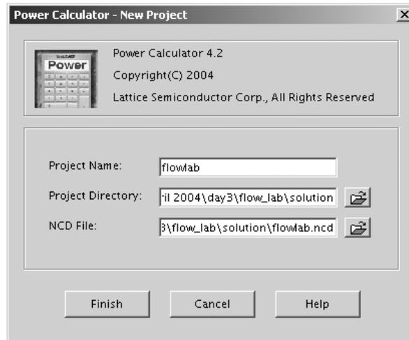
The various fields are filled in automatically with the project name the same as the ispLEVER project name and the directory also the same as the design folder. If the Post Place and Route NCD file is available, the NCD File field is also automatically filled. Users can also browse to the particular location to change the folder where they wish to create the Power Calculator project. Users can also browse to the NCD file in case it is not available at the root design folder.
