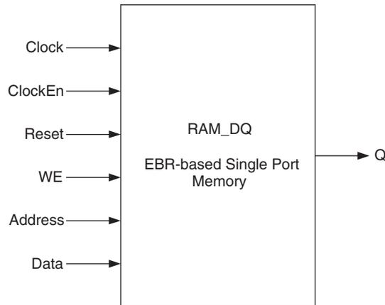
Since the device has a number of EBR blocks, the generated module makes use of these EBR blocks or primitives and cascades them to create the memory sizes specified by the user in the IPexpress GUI. For memory sizes smaller than an EBR block, the module will be created in one EBR block. In cases where the specified memory is larger than one EBR block, multiple EBR block can be cascaded, in depth or width (as required to create these sizes).
