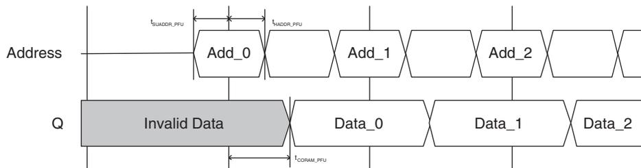
Figure 9-62. PFU Based ROM Timing Waveform – with Output Registers
