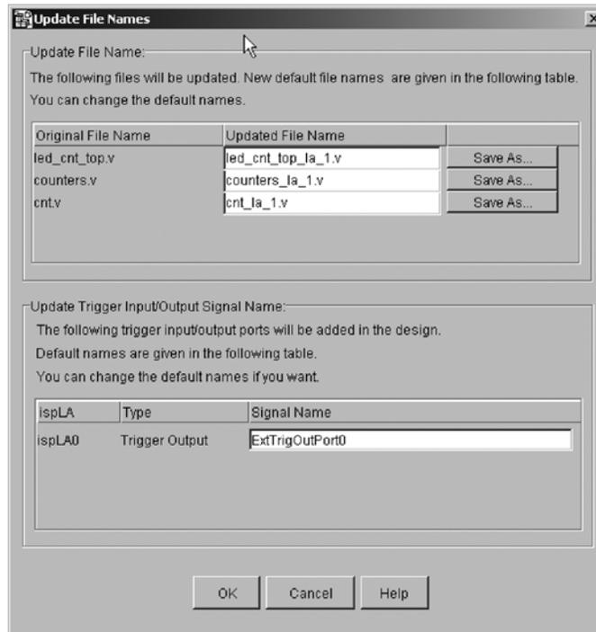
After clicking OK, you will be back in the ispTRACY Core Linker. You may now close this and return to the ispLEVER Project Navigator. At this point, it is necessary to replace the original design files with the ispTRACY Core Linker modified files. Figure 6 shows this file replacement process on a design.
