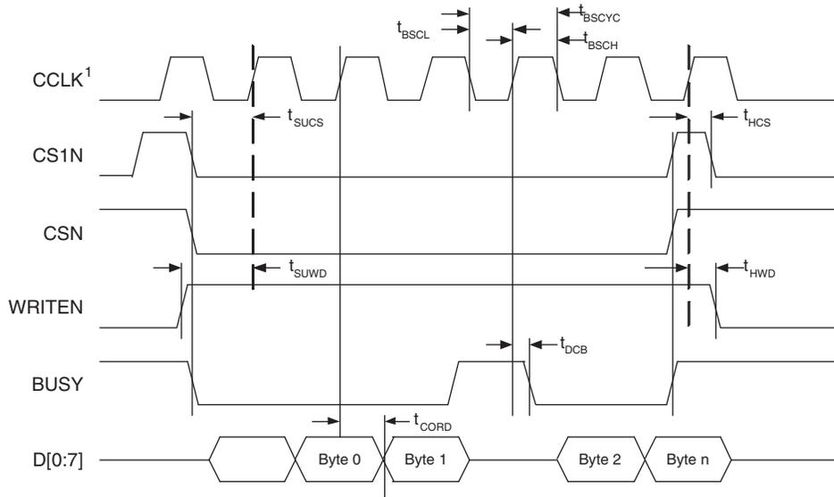
1. In Master Parallel Mode the FPGA provides CCLK. In Slave Parallel Mode the external device provides CCLK.
