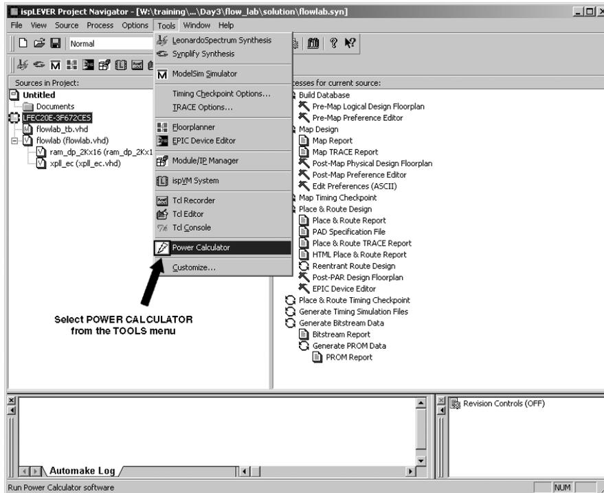
The Power Calculator does not support some of Lattice's older devices. The toolbar button and menu item is only present when supported devices are selected.
