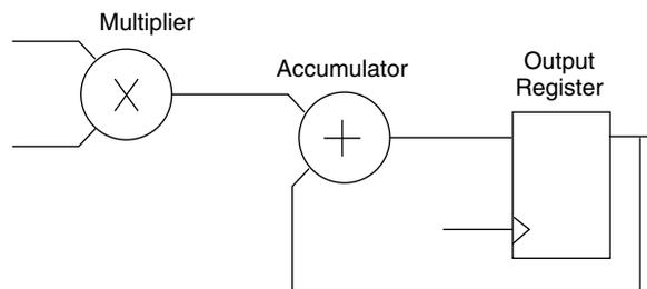
As you can see, this block diagram can be mapped directly into the sysDSP primitives. If we were to add a test point between the multiplier and the accumulator, or two output registers, the code could not be mapped into a MULT9X9MAC of a sysDSP Block. So options you could include in the design would be input registers, pipeline registers, etc. For more inferring design examples refer to EXAMPLES in your ispLEVER software.
