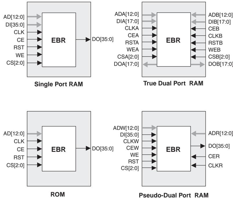
The EBR memory supports three forms of write behavior for single port or dual port operation:
