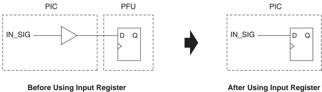
**Figure 15-12. Moving FF into PIC Output Register**
