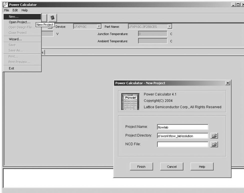
The Start Project window is used to create a new Power Calculator Project (\*.pep project). Three pieces of data are input in the Start Project window.
