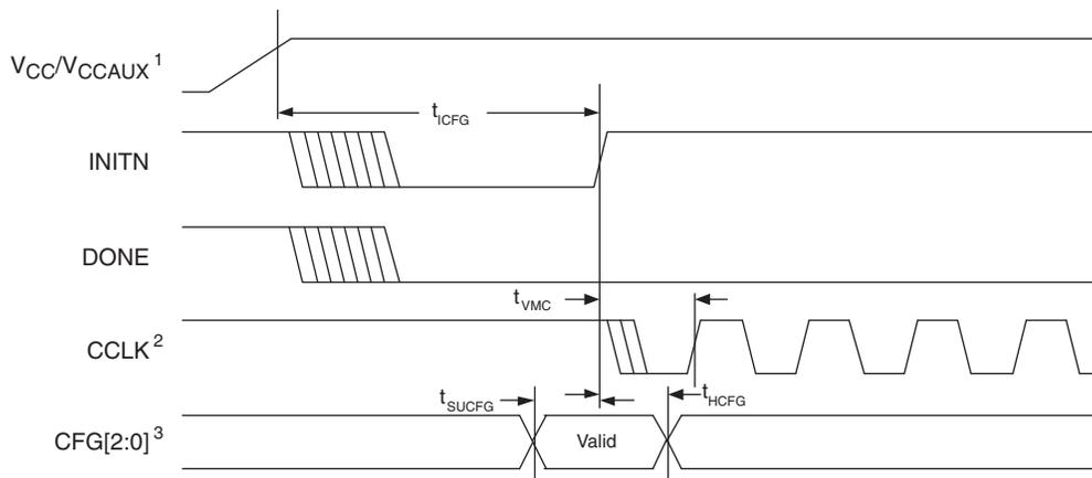
1. Time taken from  $V_{CC}$  or  $V_{CCAUX}$ , whichever is the last to reach its  $V_{MIN}$ .
