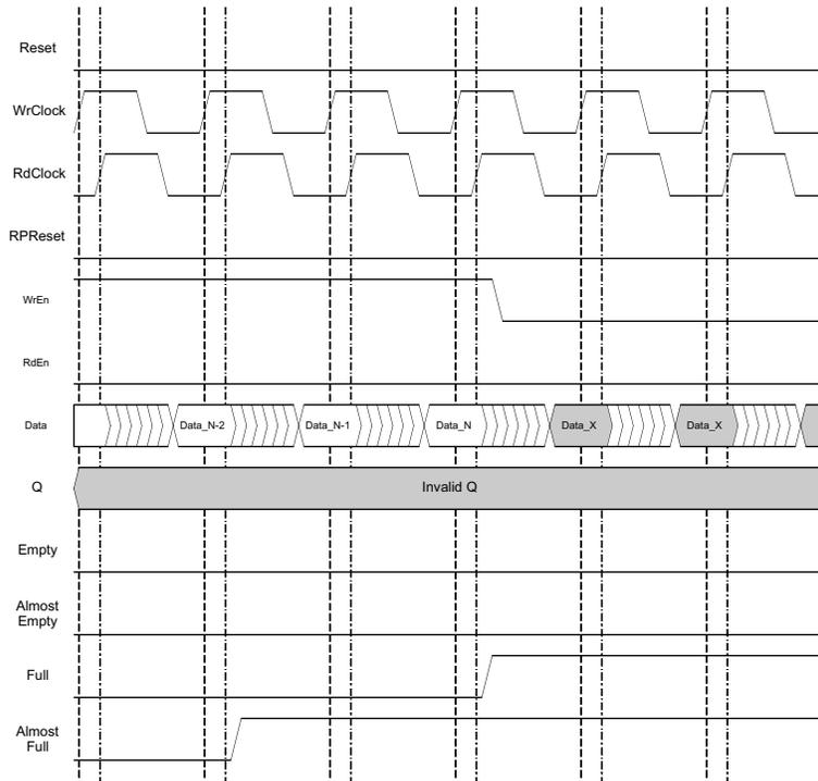
In this case, the Almost Full flag is in location 2 before the FIFO\_DC is filled. The Almost Full flag is asserted when N-2 location is written, and Full flag is asserted when the last word is written into the FIFO\_DC.
