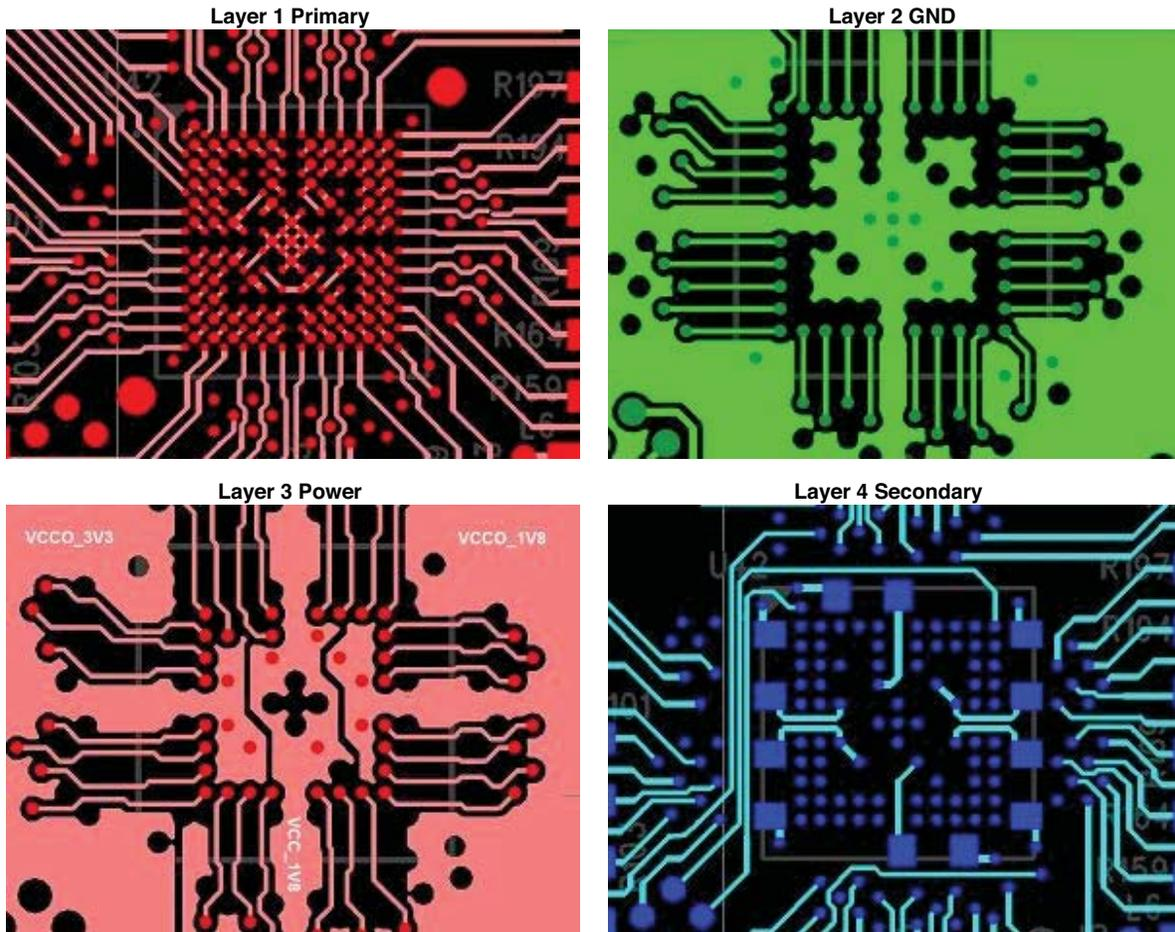
Figure 18-11. CAM Artwork Screen Shots, Example #2, 256-ball caBGA
