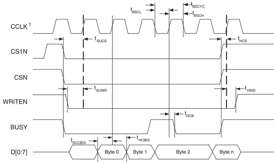
1. In Master Parallel Mode the FPGA provides CCLK. In Slave Parallel Mode the external device provides CCLK.
