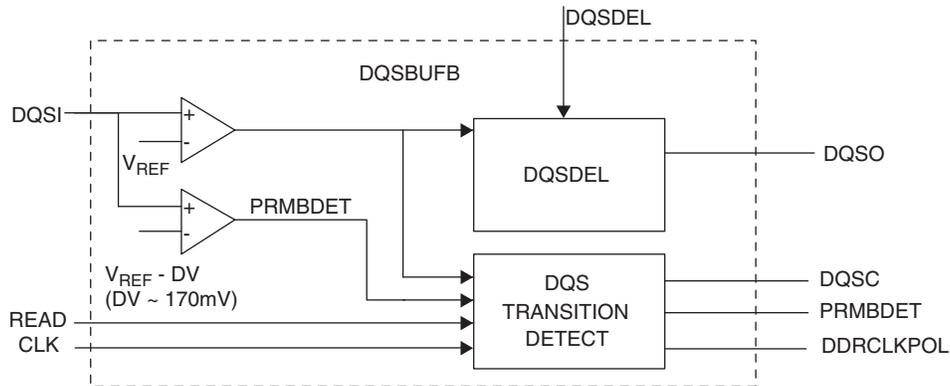
Figure 10-7 shows the primitive symbol and its ports. DQSI is the DQS signal from the memory. PRMBDET is the preamble detect signal that is generated from the DQSI input. READ and CLK are user interface signals coming from the FPGA logic. The DQSDLL block sends digital control line DQSDEL to this block. The DQS is delayed based on this input from the DQSDLL. DQSO is the delayed DQS and is connected to the clock input of the first set of DDR registers.
