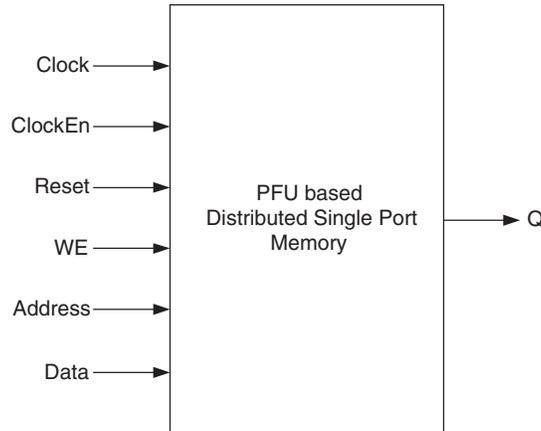
The generated module makes use of the 4-input LUT available in the PFU. Additional logic like Clock, ClockEn and Reset is generated by utilizing the resources available in the PFU. The basic Distributed Single Port RAM primitive for the LatticeECP/EC and LatticeXP devices is shown in Figure 9-52.
