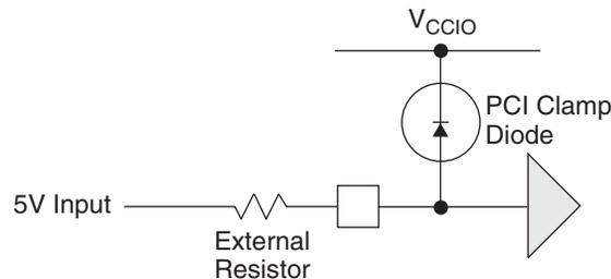
The value of this external resistor will depend on the PCI clamp diode characteristics. You can find the voltage vs. current data across this diode in the device IBIS model.
