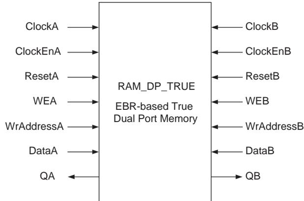
The generated module makes use of the RAM\_DP\_TRUE primitive. For memory sizes smaller than one EBR block, the module will be created in one EBR block. In cases where the specified memory is larger than one EBR block, multiple EBR blocks can be cascaded, in depth or width (as required to create these sizes).
