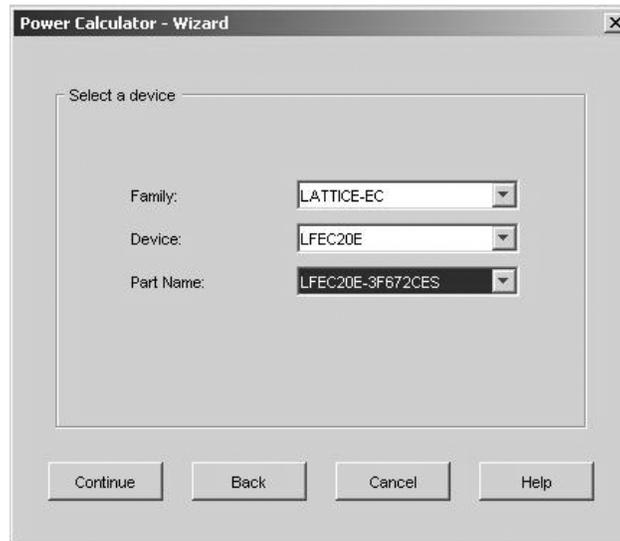
In the following screens, as shown in Figures 12-8-12-12, users can select further resources such as I/O types and provide a clock name, frequency at which the clock is running and other parameters, by selecting the appropriate resource using the pull-down Type menu:
