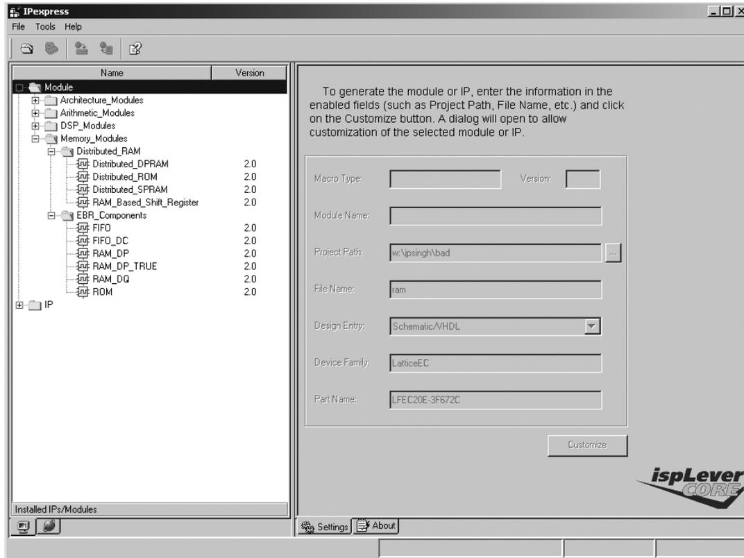
The left pane of this window has the Module Tree. The EBR-based Memory Modules are under the **Module > Memory- Module > Distributed RAM and EBR\_Components** and the PFU-based Distributed Memory Modules are under **Storage\_Components** as shown in Figure 9-4.
