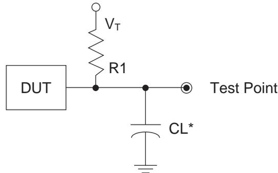
\*CL Includes Test Fixture and Probe Capacitance
