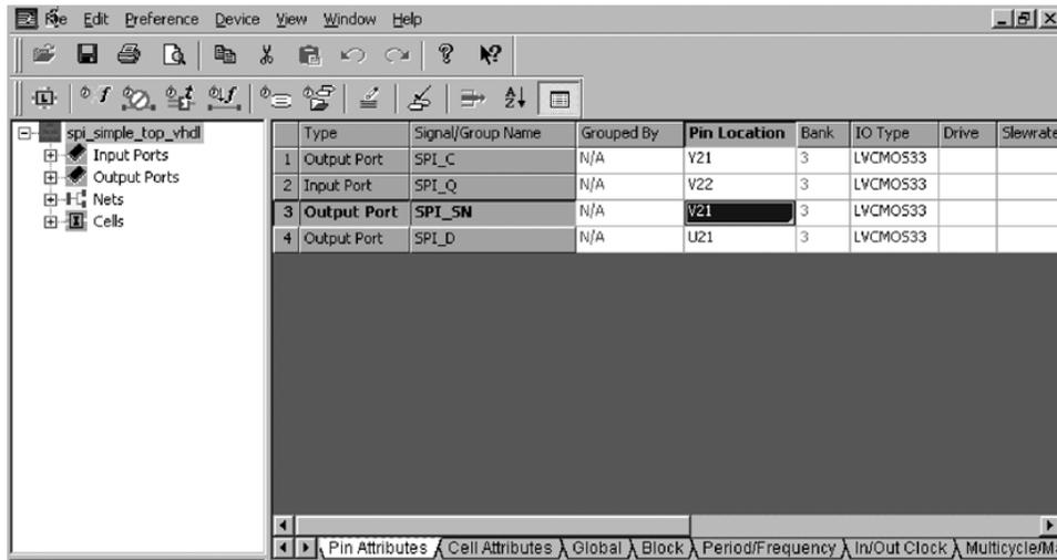
After all of the pin attributes have been entered, close the Preference Editor, scroll down the right window, and double click on Generate Bitstream Data (see Figure 21-17). Once the bitstream has been generated, go to the Programming Procedure section of this document.
