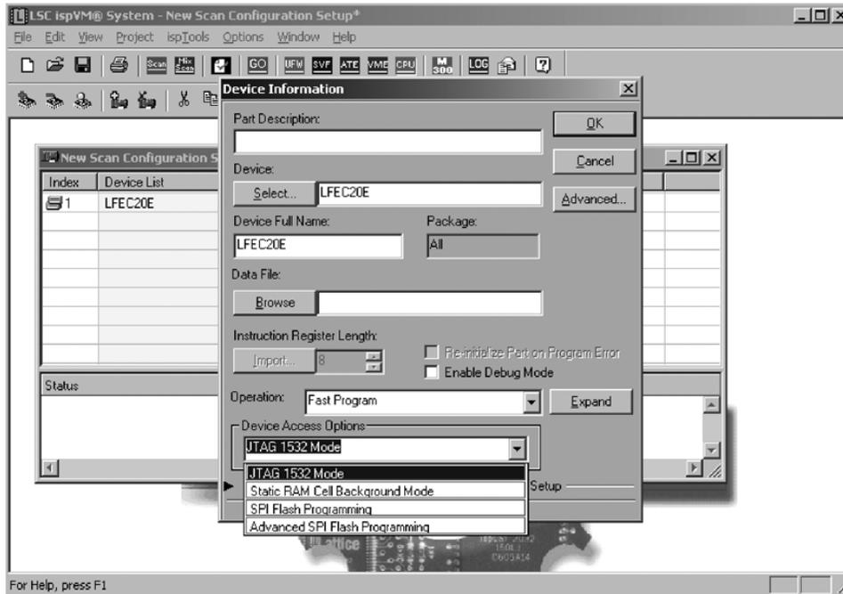
5. Under **Device Access Options**, select either **SPI Flash Programming** or **Advanced SPI Flash Programming**. To use the default Soft IP and program the SPI Serial Flash with a single LatticeECP/EC bitstream, select **SPI Flash Programming**. If the Soft IP was instantiated into your design, or if you need to merge multiple bitstreams into a single SPI Serial Flash device, select **Advanced SPI Flash Programming**.
