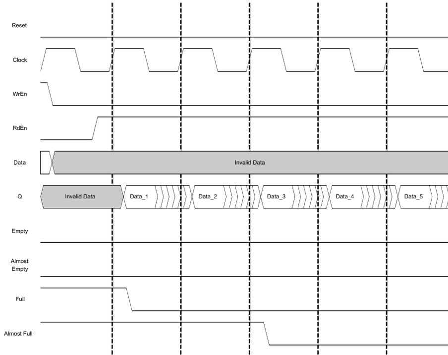
Similarly as the data is read out, and FIFO is emptied, the Almost Empty and Empty flags are asserted. Below is the
