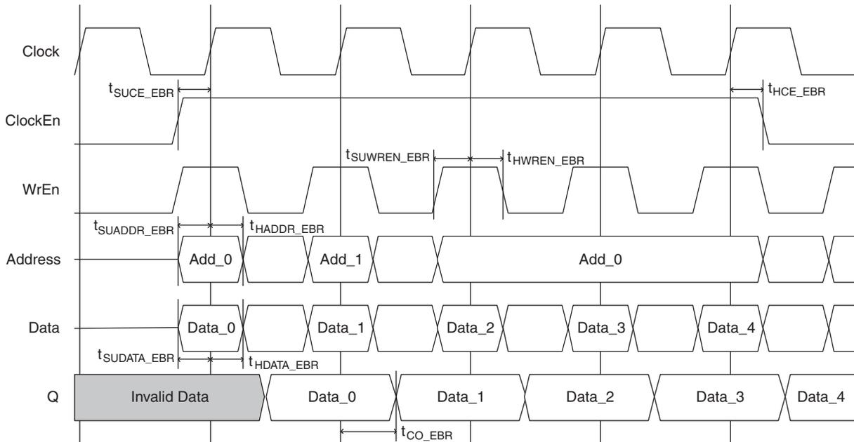
Figure 9-14. Single Port RAM Timing Waveform – WRITE THROUGH Mode, with Output Registers
