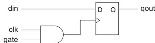
**Figure 15-10. Synchronous: Clock Enabling**
