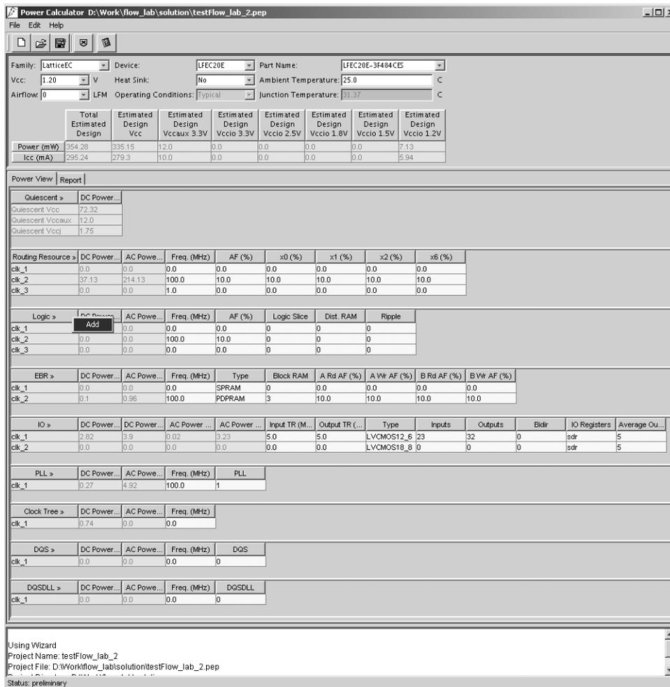
This adds a new row for the logic resource utilization with clock domain as clk\_1.
