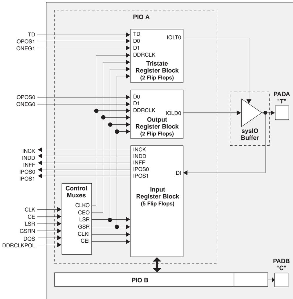
Two adjacent PIOs can be joined to provide a differential I/O pair (labeled as “T” and “C”) as shown in Figure 2-25. The PAD Labels “T” and “C” distinguish the two PIOs. Only the PIO pairs on the left and right edges of the device can be configured as LVDS transmit/receive pairs.
