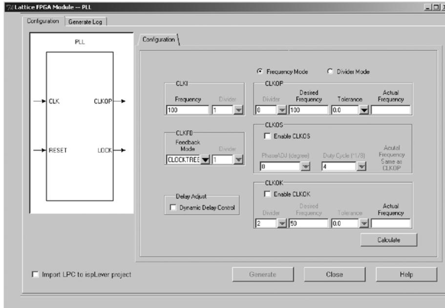
**Divider Mode:** In this mode, the user sets the input frequency and divider settings. It is assumed the user is familiar with the PLL operation. The user must choose the CLKOP Divider value to maximize the  $f_{VCO}$  to achieve optimum PLL performance. After input frequency and divider settings are set, clicking the 'Calculate' button will display the output frequencies. If the divider settings are out of the PLL specification, the software will generate an error.
