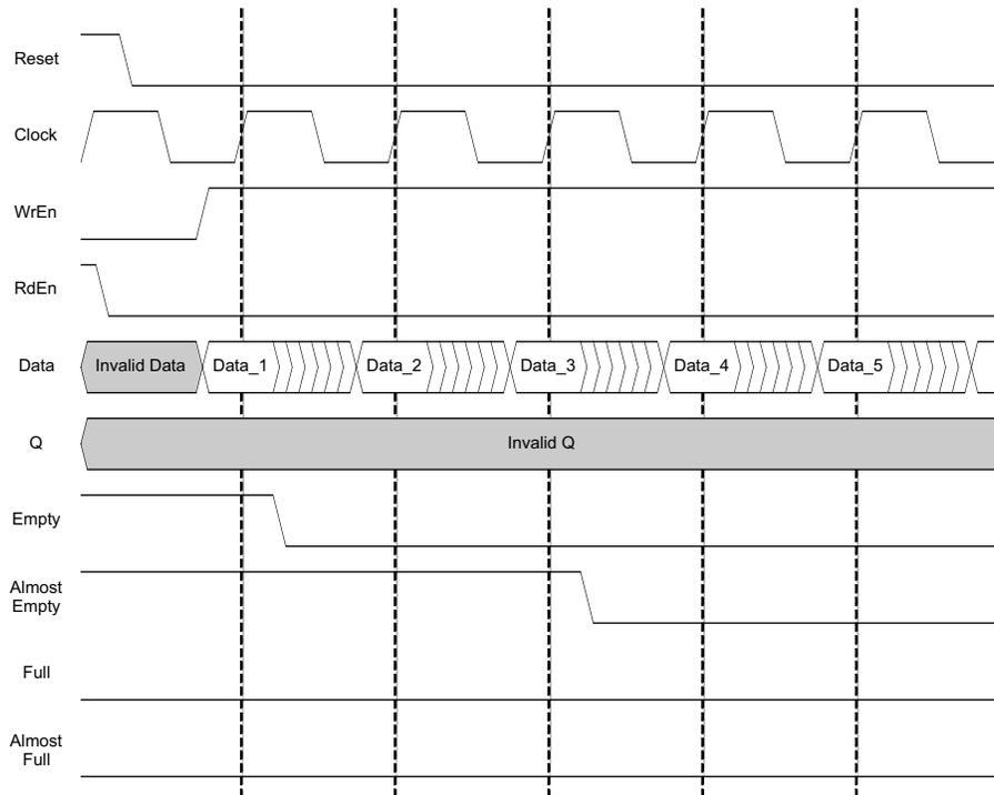
**Figure 9-38. FIFO with Output Registers, End of Data Write Cycle**
