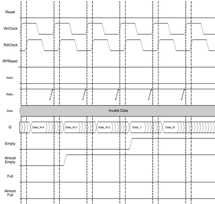
Finally, if you select the option enable output register with RdEn, it still delays the data out by one clock cycle (as compared to the non-pipelined FIFO\_DC), and the RdEn should be high also during that clock cycle. Otherwise the data takes an extra clock cycle when the RdEn is goes true.
