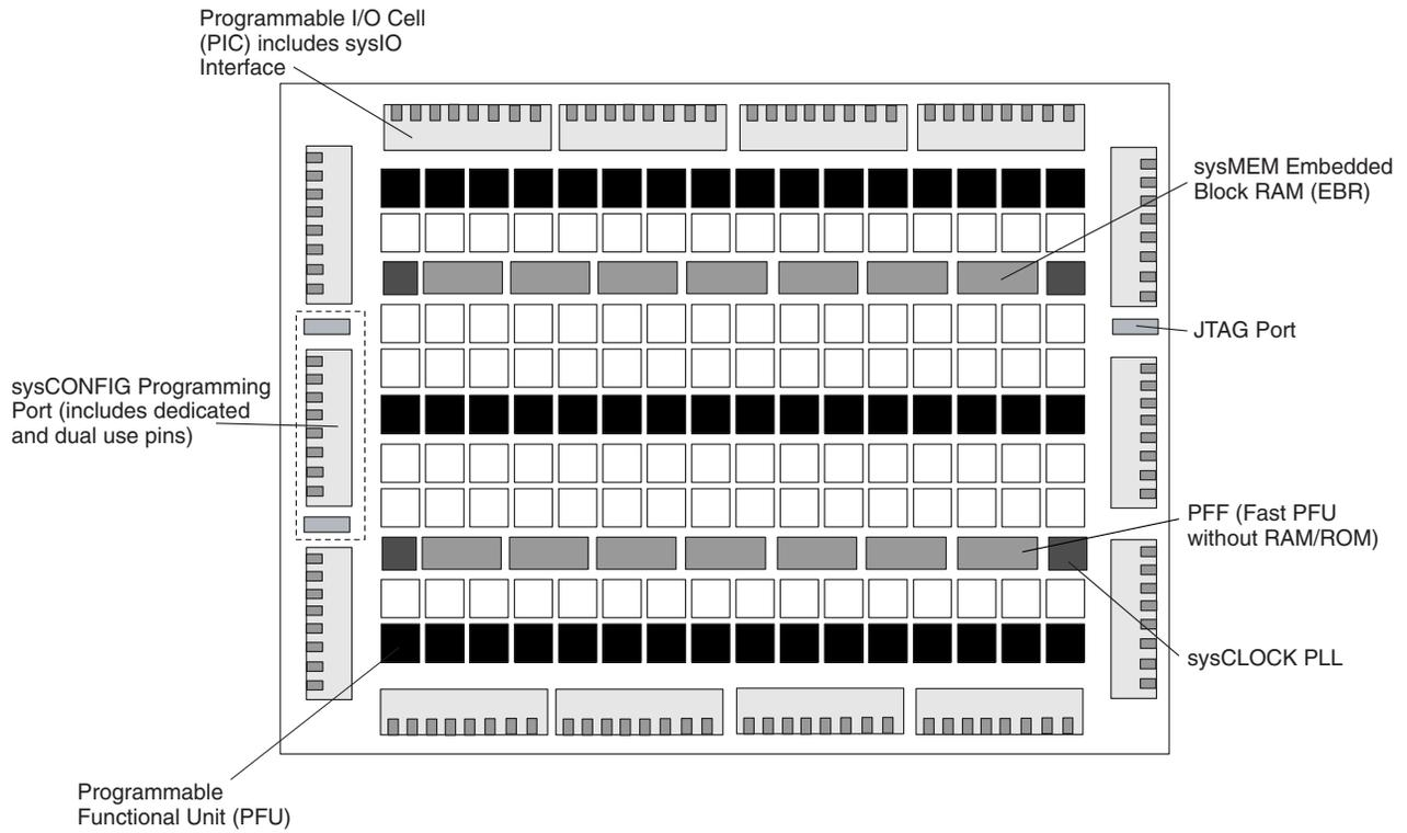
**Figure 9-2. Simplified Block Diagram, LatticeECP Device (Top Level)**
