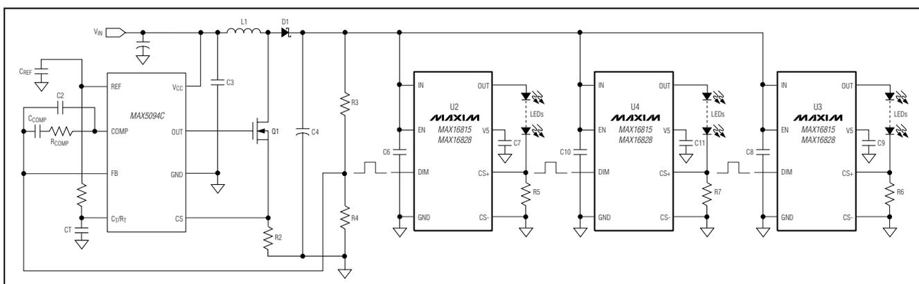
Figure 5. Multichannel HB LED Drivers for LCD Backlight
