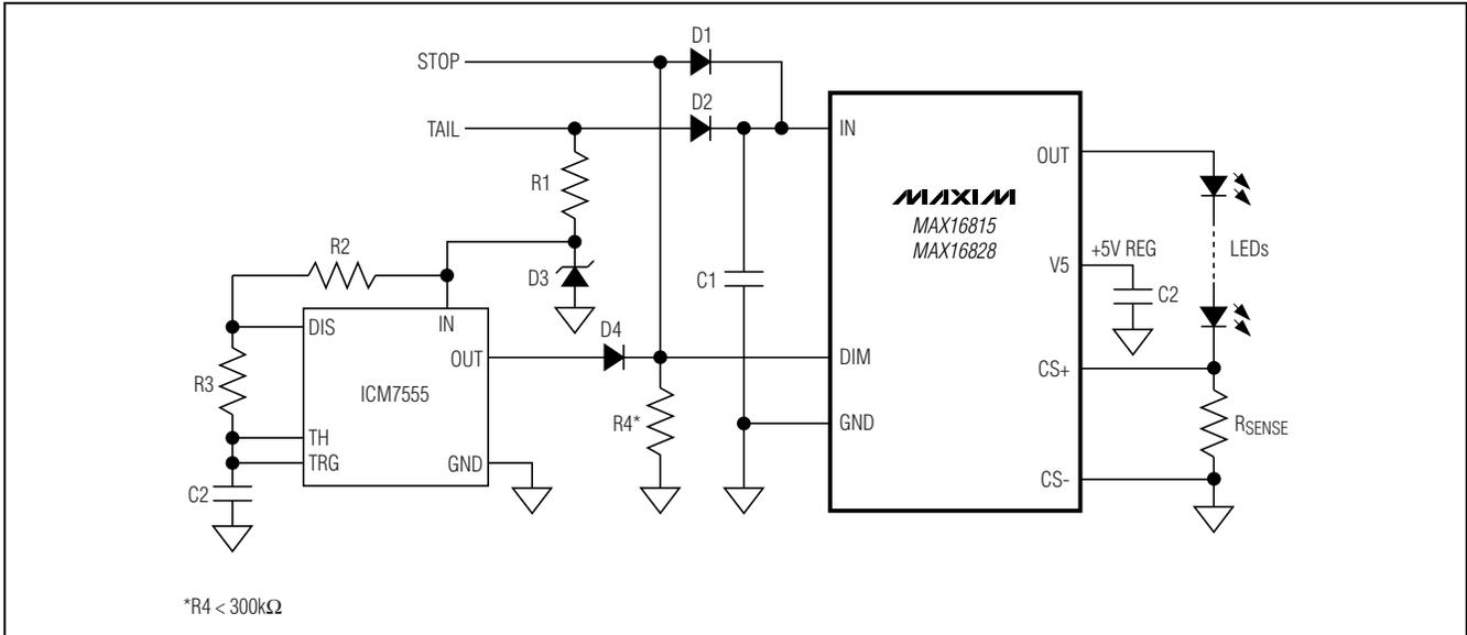
Figure 1. PWM Dimming Operation with ICM7555 Timer
