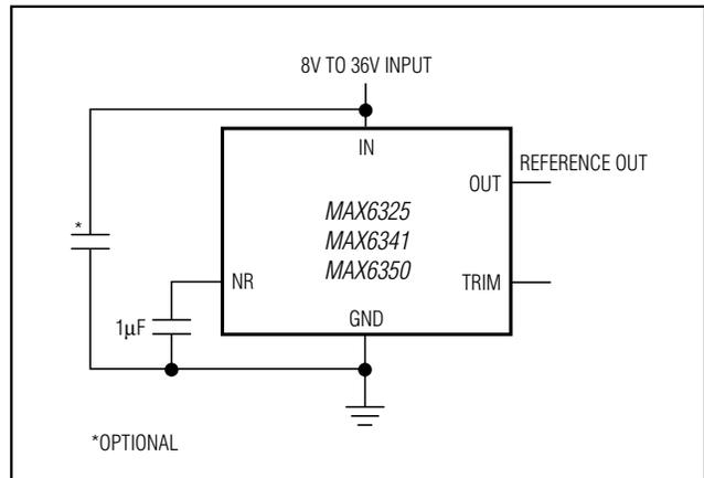
Figure 2. Noise-Reduction Capacitor
